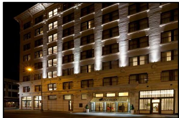
*This building utilizes up-lighting, under-eave lighting, and clear-story lighting to provide a nighttime setting for the building.*
