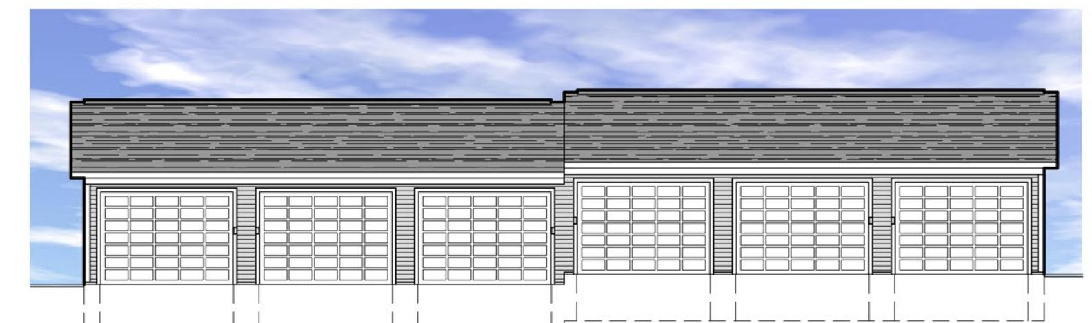
6-Stall Front Elevation w/ 2 Finish Floor Elevations
