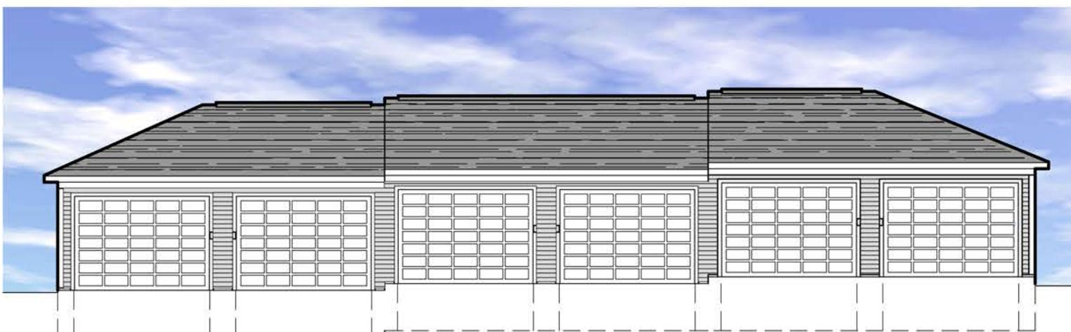
6-Stall Front Elevation w/ 3 Finish Floor Elevations
